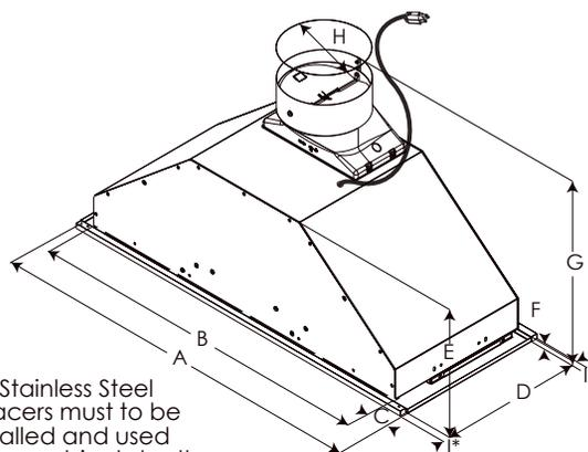
I\* - Stainless Steel Spacers must to be installed and used when cabinet depth is greater than 12".
